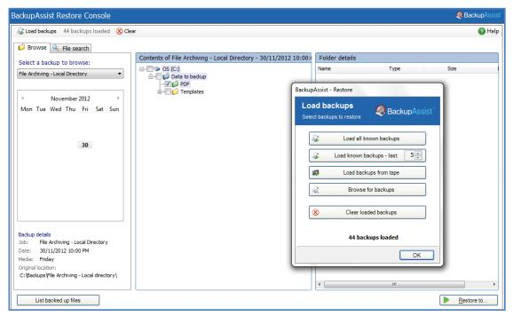
Figure 4: BackupAssist Restore Console – backup and data selection
