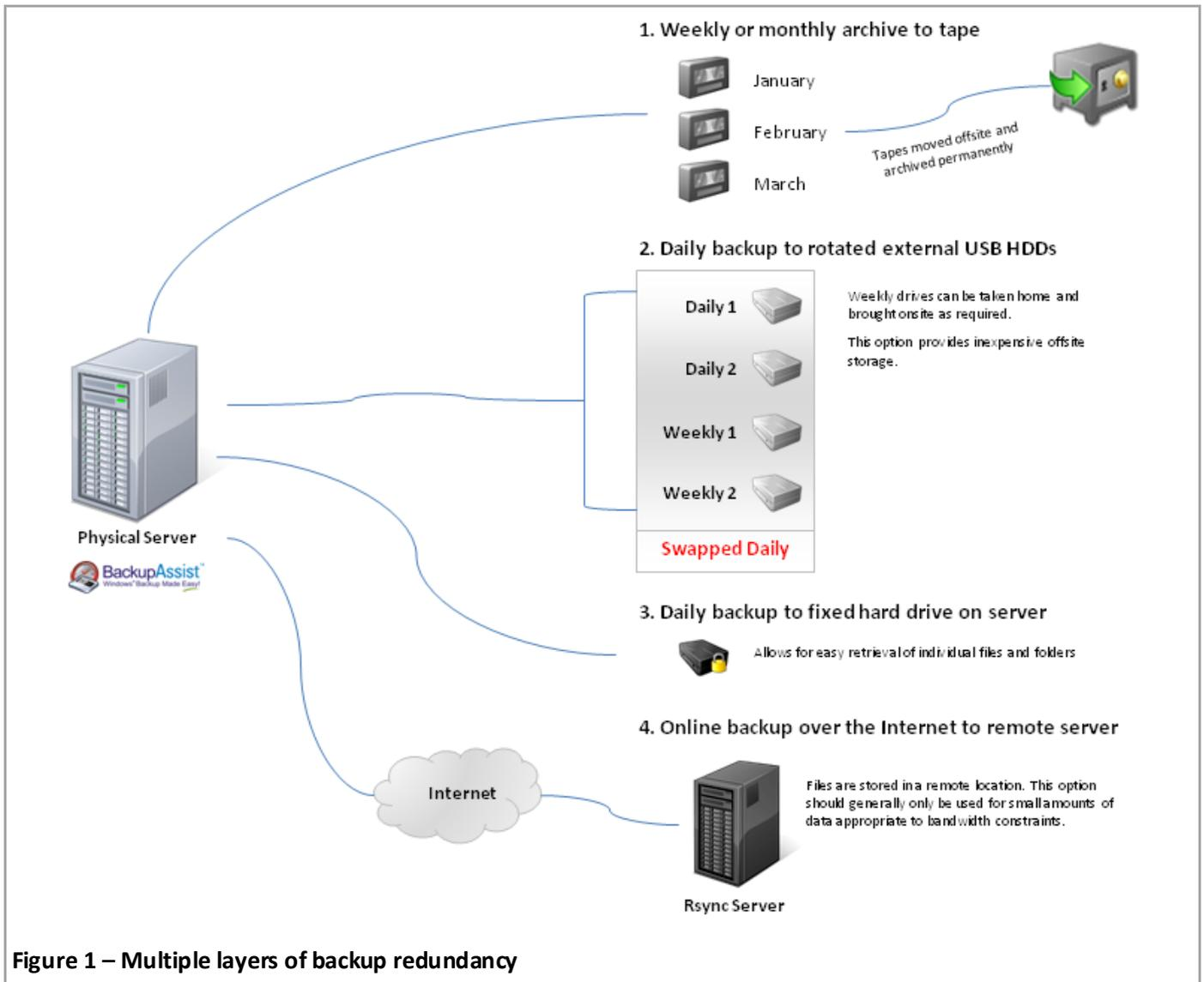
Figure 1 – Multiple layers of backup redundancy
